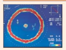
The full circle scan helps to detect fish schools at any bearing, all around the vessel.
