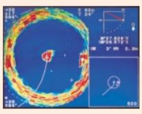
Own ship track is monitored with respect to the sonar sounding area. An Unrivaled feature for purse seining or bottom trawling.
