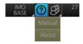
On the [About] screen, click the [Version] tab to show the ECDIS software version no., conning software version no., S52 presentation library version, ENC user permit no., and C-MAP SDK software version no. Click the [System] tab to show ECDIS system information: CPU type, RAM capacity, SSD free/SSD capacity and Unified ID.
