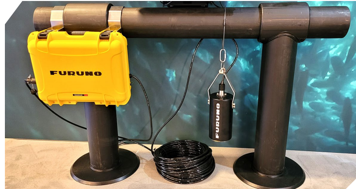
The echo sounder and edge processing unit are placed in a waterproof casing and attached to the pen.
