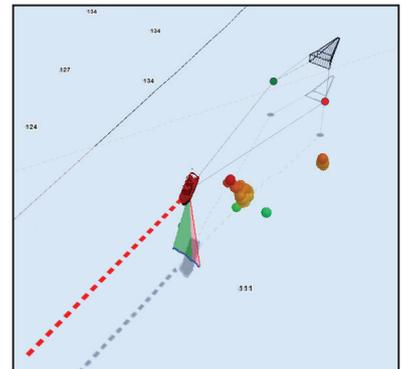
Combined with a compatible multi-beam sounder, TZ Professional will literally display the fish entering the trawl thanks to our amazing 2D/3D Fish Targets display.
