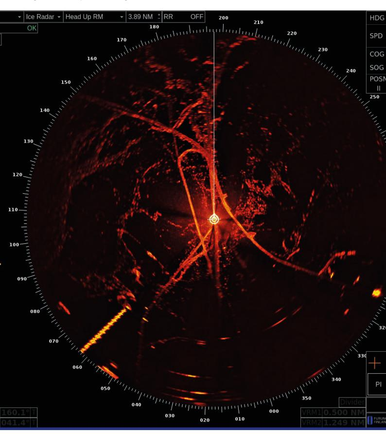
Equalize feature visualizes ice radar picture with adjusted brightness ratio both on center and near edge of display:
