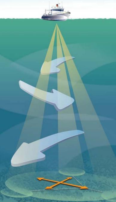
The FURUNO CI-88 is a Doppler Sonar Current Indicator designed for every type of fishing vessels and hydrographic survey vessels. The high-definition 10.4" color LCD continuously presents tide speed and direction at three depth layers simultaneously in addition to ship's speed and drift. This variety of current information allows you to predict net shape and plan when to throw your net.
