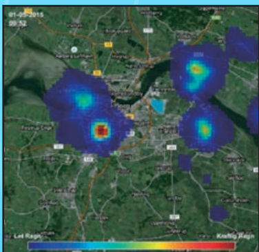
High intensity hailstorm over the city of Aalborg. Resolution is 300 x 300 meter. Background map, Google Map, 2015
